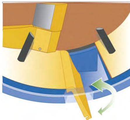
The mixer is equipped with an integral self cleaning mechanism:
